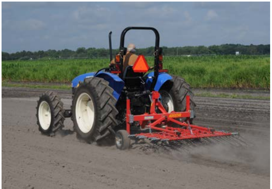
Figure 4. Shallow cultivation with a tine weeder to prepare a stale seed bed for planting.
